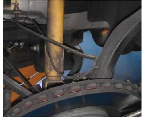
**5** Remove bottom strut bolt with 18 mm.
