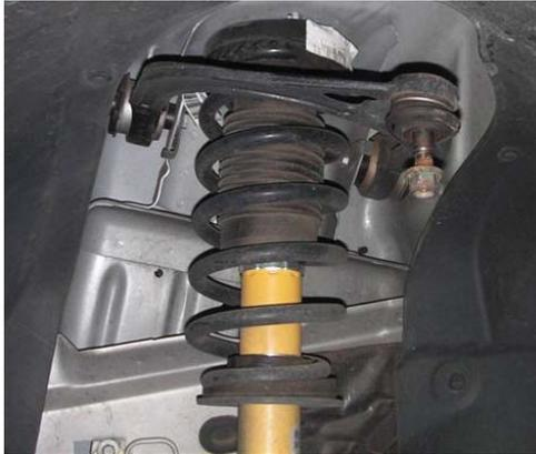
**4** Remove sway bar nut from strut with 21 mm and hold with 10 mm.
